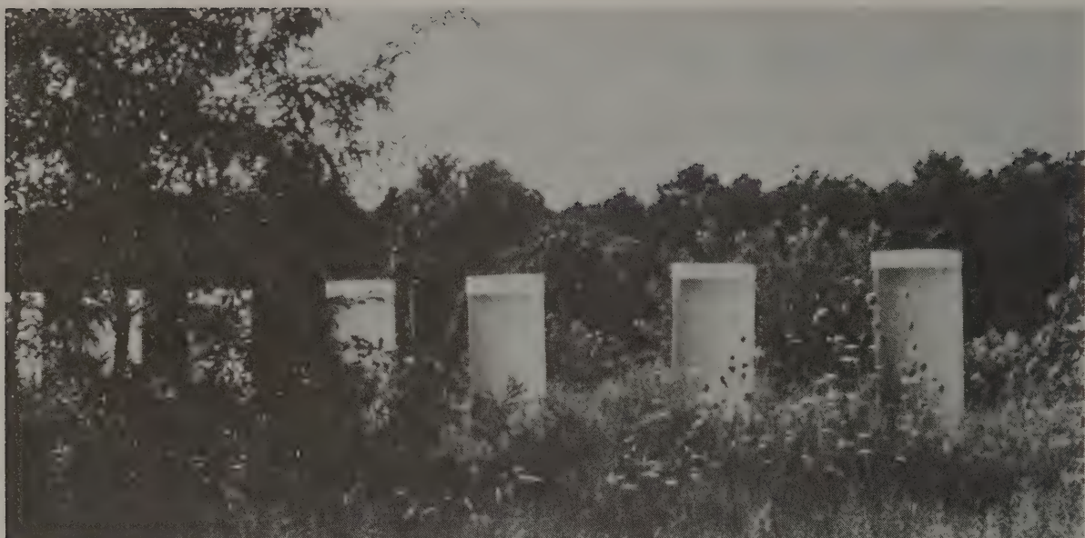
Solar tubes, 18" diameter, 5' high, housing algae and tilapia feeding experiments.
